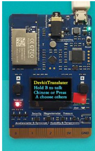
Figure 16-28. MXChip IoT DevKit that is wi-fi connected and running an Azure-based translator project found integrated with VSCode Azure IoT Tools extension. Source: https://microsoft.github.io/azure-iot-developer-kit/docs/projects/
