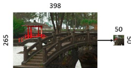
Figure 16-3. An image is resized from 398×265 pixels to 50×50 pixels. Often in ML, an image must be resized before using in algorithms because the algorithms usually expect consistently sized inputs
